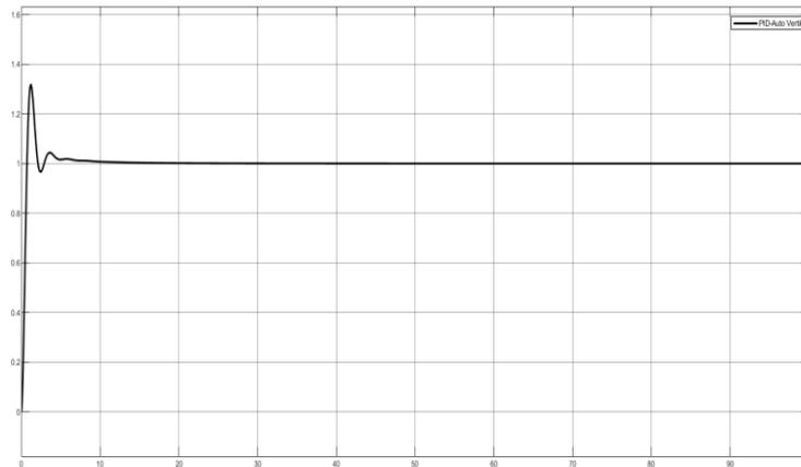
Figure 7. PID auto-tuning for vertical axis
