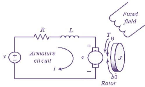
Figure 1. Schematic diagram of a DC motor
