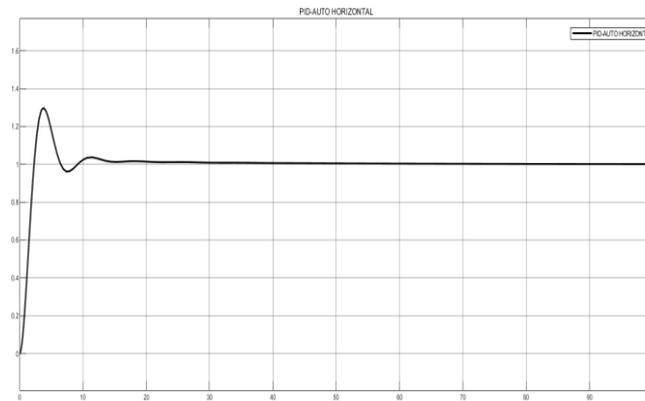
Figure 6. PID auto-tuning for horizontal axis
