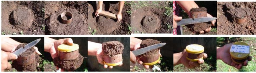
Figure 2. Illustration of soil sampling procedures for soil fertility assessment and fertilizer recommendation development.
